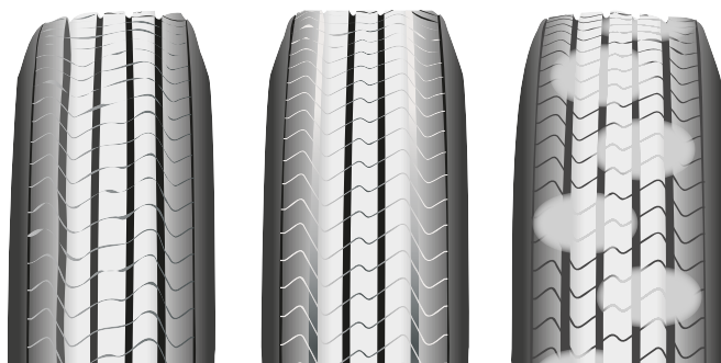
Figure 219: Feathered, Edge Wear, Cupped Wear Patterns
