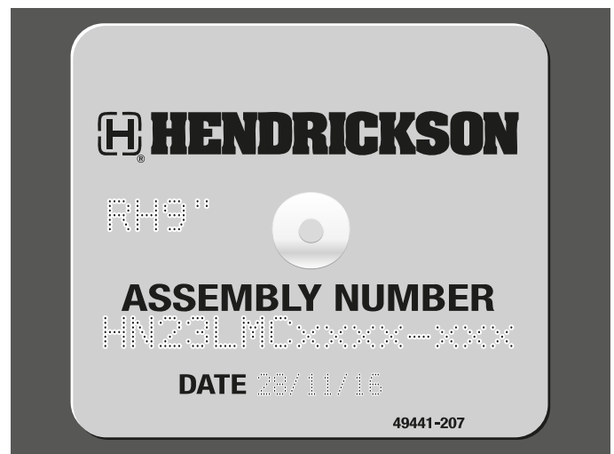
Figure 16: Axle Assembly Number Plate
