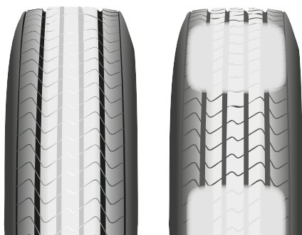
Figure 218: Centre Wear & Flat Spot Tyre Wear Patterns
