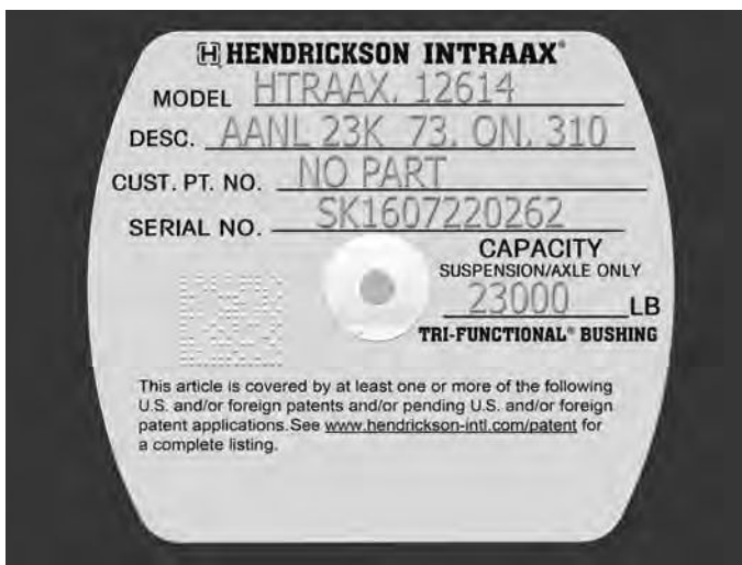
Figure 15: Axle Identification Number Plate
