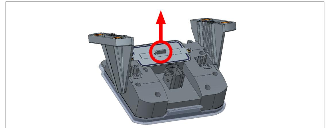
3. Remove the battery cover with a pair of flat nose pliers.
