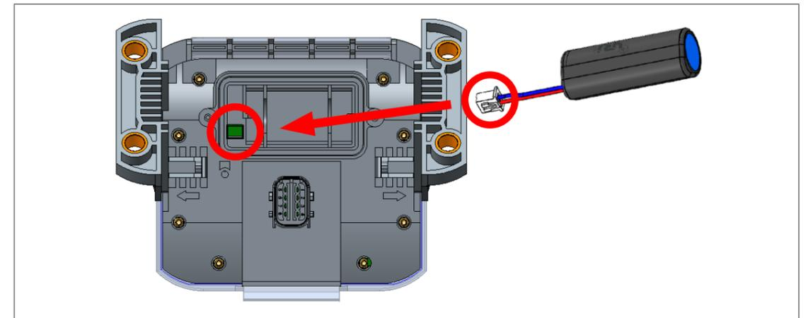
5. Push the replacement battery plug into the slot provided for it with the correct polarity and insert the replacement battery.
