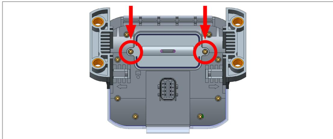
2. Unscrew the two Torx® screws on the battery cover.
